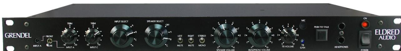
**Input A:** First up on the Grendel front panel is an additional 3.5mm stereo input socket for INPUT A and next to this a switch that selects either this socket or the rear panel RCA Input A connections. The 3.5mm socket is perfect for connecting portable audio devices such as smartphones, mp3 players, or tablets.
